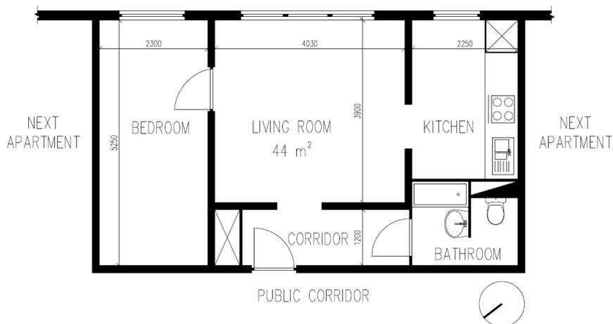
**Fig. 1:** Floor plan of the apartment, Ostrava, Czechia [12]
